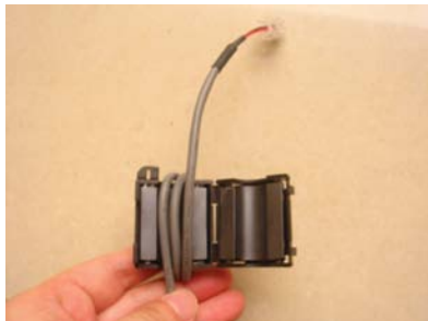
Fig.28 Connection Manner of Crystal Connector, Communication Line and Magnetic Ring
