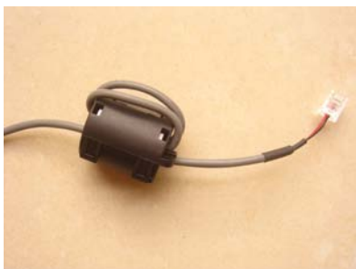
Fig.29 Connection Location of Crystal Connector, Communication Line and Magnetic Ring
