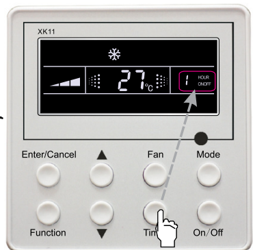
Fig.10 Timer setting under on state of the unit
