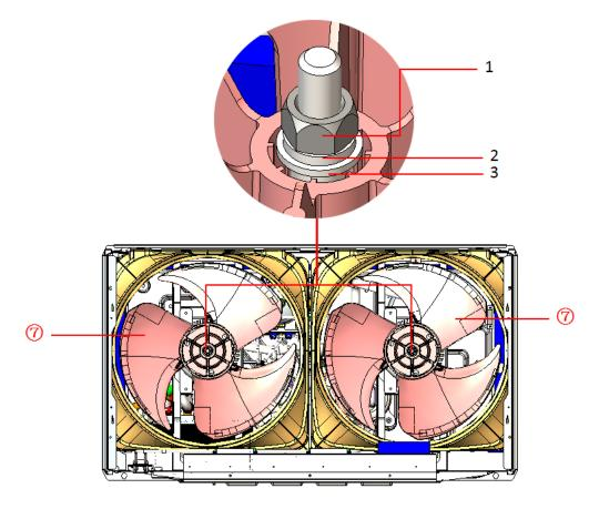
1 - nut; 2 - spring washer; 3 - flat piece;  $\bigcirc$  - blade.
