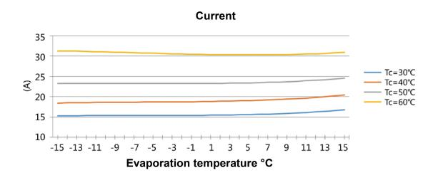
When the compressor frequency is 120 Hz, the current curve corresponding to the evaporation temperature and condensation temperature is shown as follows:
