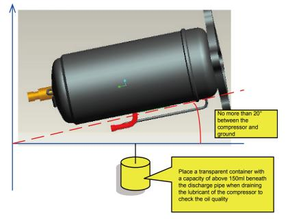
3 Place the collected compressor oil in a bright place to check if it contains impurities and discolors, and smell the compressor oil. Normal lubricant has no obvious pungent odor.
