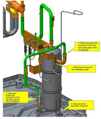
2) Checking gas-liquid separator
