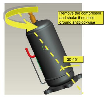
2 Place the compressor at a position above the level of the ground, pour oil from the compressor exhaust port, and use a beverage bottle or other transparent container (with a volume of over 150 ml) to store oil.
