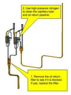
2 Checking the liquid pipe filter.
