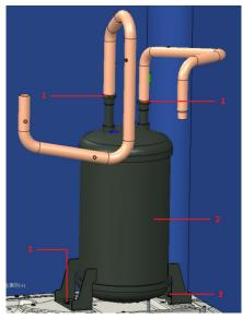
1 --- Connection points 2 --- Gas-liquid separator 3 --- Bolts and washers
