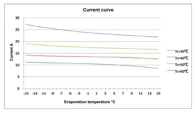
When the compressor frequency is 60 Hz, the current curve corresponding to the evaporation temperature and condensation temperature is shown as follows:
