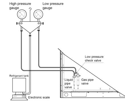
Step 2: Fully open the liquid pipe valve and gas pipe valve of each module.
