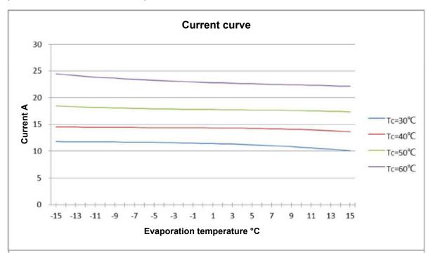
When the compressor frequency is 90 Hz, the current curve corresponding to the evaporation temperature and condensation temperature is shown as follows:
