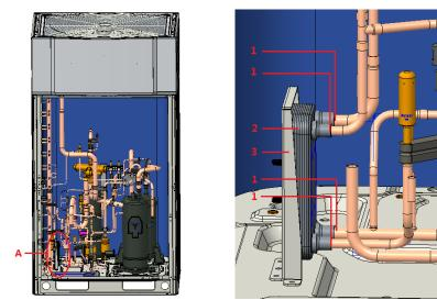
A --- plate heat exchanger assembly
