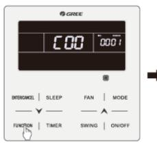
Long press FUNCTION for five seconds when the conditioner is on or off to view parameters.
