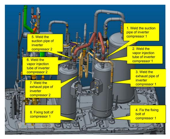
Before replacing the compressors, make sure that the models of the compressors to be replaced are same as the models of the new compressors. The new compressors must be installed at the same places of the respective old compressors and wired correctly. We recommend you replace the compressors one by one.
