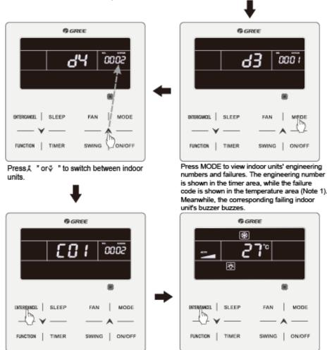
Press ENTER/CANCEL (Note 2) to quit the interface of the indoor unit's engineering number and failure and return to the previous interface.
