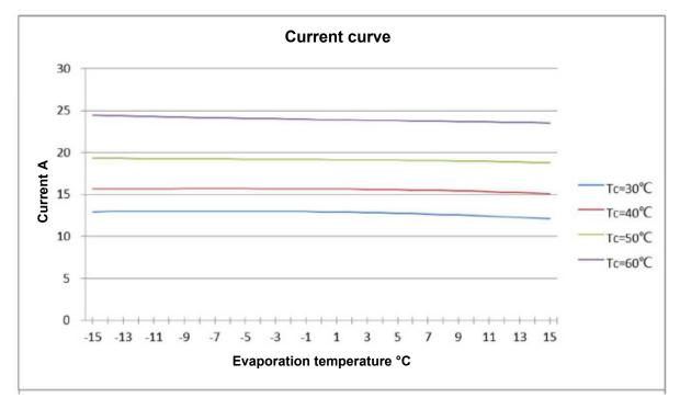
When the compressor frequency is 120 Hz, the current curve corresponding to the evaporation temperature and condensation temperature is shown as follows:
