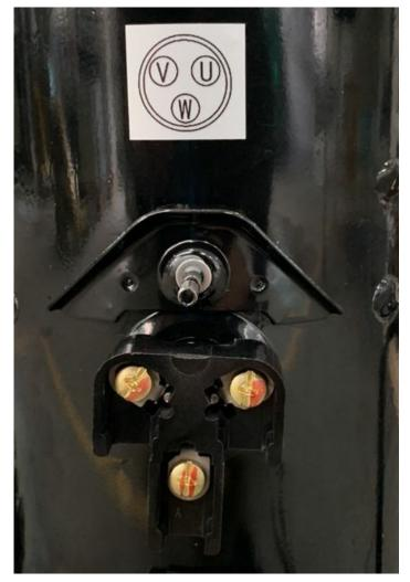
Measure the grounding resistance of each wiring terminal, which should be greater than 10 M $\Omega$ ; otherwise, the compressor has an internal fault.
