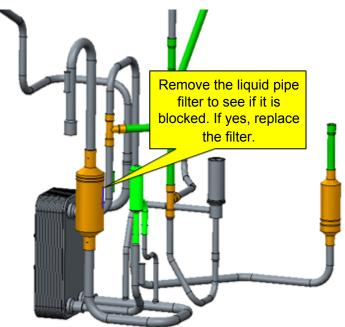
Remove the other piping components according to the actual conditions. If the components are not replaced immediately after removing the pipeline, use tape to seal the pipeline to prevent moisture and impurities from contaminating the system.
