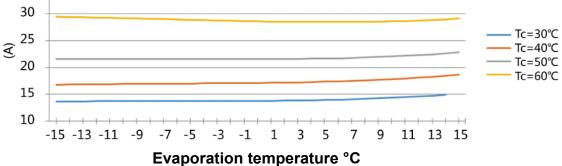
When the compressor frequency is 90 Hz, the current curve corresponding to the evaporation temperature and condensation temperature is shown as follows:
