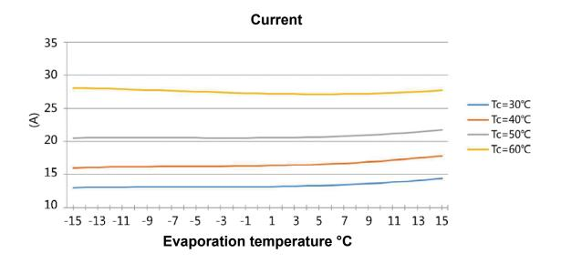
When the compressor frequency is 60 Hz, the current curve corresponding to the evaporation temperature and condensation temperature is shown as follows:
