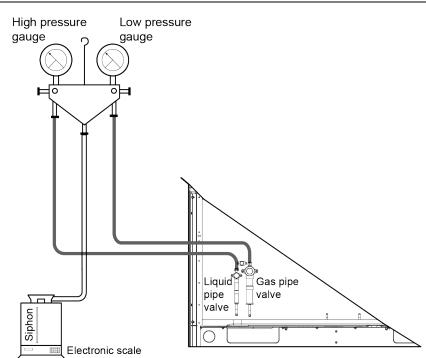
**Step 5:** Open the high pressure gauge valve (the low pressure gauge valve remains closed), charge the system with refrigerant, and record the weight change of the refrigerant tank.
