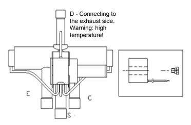
Marks are made on the 4-way valve: D indicates connection to the exhaust side, E indicates connection to the IDU evaporator, S indicates connection to the air inlet of gas-liquid separator, C indicates connection to the condenser; when the system runs in the cooling mode, C indicates that the
