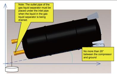
It is also necessary to use a transparent container to hold the impurities in the gas-liquid separator, observe the impurity color and seal the container, and return it to the factory to check the impurity composition.
