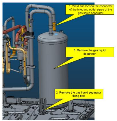
After removing the gas-liquid separator, check whether the gas-liquid separator contains impurities or other substances. The checking procedure is described as follows:
