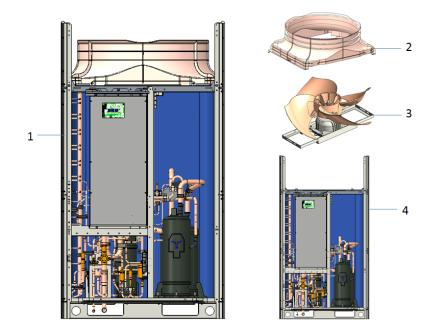
(2) Remove the electrical appliance box: Use a screwdriver to remove the screw that secures the electrical appliance box and remove the electrical appliance box 2. Note: Before removing, loosen the two refrigerant tubes of the electrical box radiator.
