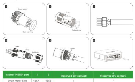
INV-meter connection meter side, INV and meter connected by RS485 2pin cable.
