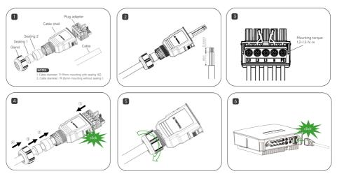
• Step7: Insert the block into AC connector, as shown in the figure below.
